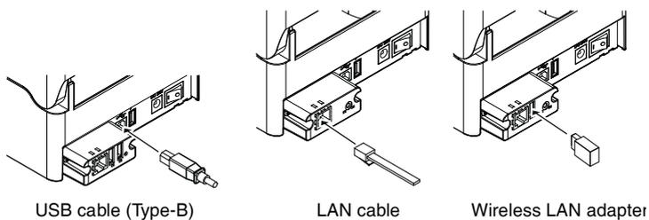
**3. Insert the other end of the cable into the appropriate interface port in the host computer.**
