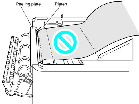
6. Pull down the backing paper further, so that it extends at least 7 cm from the peeler cover (illustration A).
