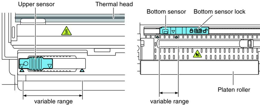
The range of bottom sensor and upper sensor horizontal adjustment is 10 steps between the triangle marks (▲).
