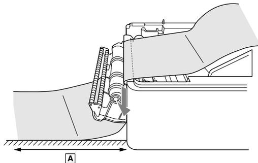
**7. Make sure the media is in abutment with the left media guide and then adjust the position of the right media guide in accordance with the media width.**
