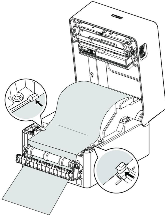
At this time, check that the label is not over the bottom sensor or fed past the bottom sensor (check that only the backing paper passes the bottom sensor).
