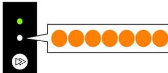
**3. Press and hold the FEED key for at least 3 seconds.**
