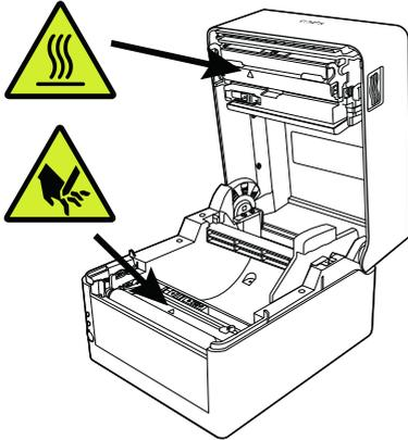
These labels indicate that the head becomes hot, so touching it may cause burns, and touching the auto cutter and manual cutter when opening the paper cover may cause cuts on hands.
