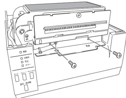
**Note** To prevent the cutter stand unit from being attached in a tilted position, fix it by pressing it against the underside.
