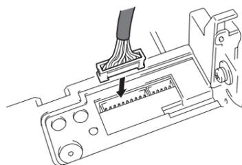
**Note** Make sure that the connector is inserted all the way in.
