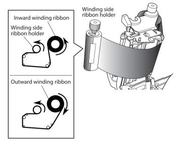
6. Set the ribbon holder on which the paper core has been set in the ribbon drive unit, then rotate it in the direction shown by the arrow to remove slack and wrinkles from the ribbon.
