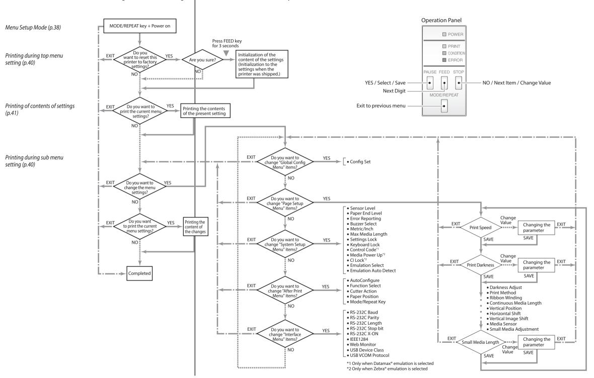
This particular example is changing the print speed and print darkness then continues through the remainder of the "Print Setup" menu. The actual output from the printer is "vertically reversed" due to the way the printer outputs the menu options. Please look at the example below to see how the output changes.
