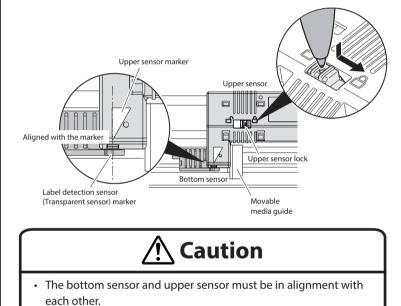
• Attempting to move the sensor while still locked may damage it.
