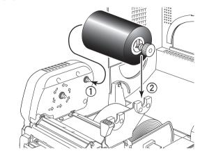
4. Push the large blue-head open lever to release the head unit. Pull out the ribbon from the bottom of the head unit to the ribbon winding side.
