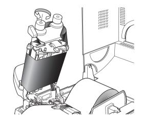
Ribbon Tension Adjustment (p.55) Ribbon Balance Adjustment (p.56) 7. Push the head close knob to lower and lock the head unit. Be sure to always push the head close knob to lock the head unit. If the ribbon is wrinkled, push the FEED key until the wrinkles disappear. If the wrinkles do not disappear or if it slips, perform ribbon balance adjustment and ribbon tension adjustment. See "Chapter 3 Printer Adjustments" for these adjustment methods.
