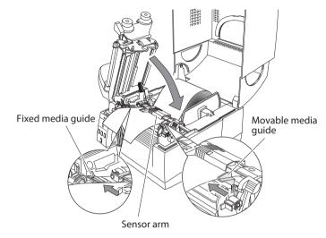
9. Push the head close knob to lower and lock the head unit. Be sure to always push the head close knob to lock the head unit. Align it with the width of the media that has been set, then set the media width and media thickness adjustment dials. See "Chapter 3 Printer Adjustments".
