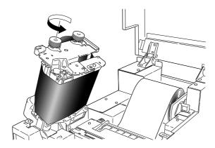
Lower the head unit back down to the closed position. Push the head close knob firmly to close and lock the mechanism.
