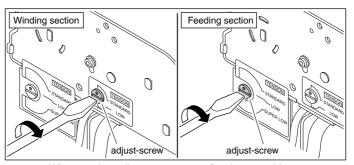
When turning adjust-screw, use a flat-tip screwdriver.
