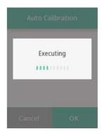
4. If the automatic adjustment is completed normally, "OK" will be displayed on the screen. If it is completed abnormally (adjustment not possible), the error LED flashes, and "Failed" will be displayed on the screen.
