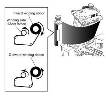
5. Set the ribbon holder on which the paper core has been set in the ribbon drive unit, then rotate it in the direction shown by the arrow to remove slack and wrinkles from the ribbon.
