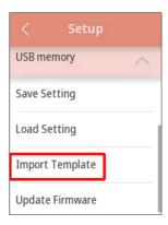
3. Press the "OK" button at the bottom of the screen to import the template from the USB memory.
