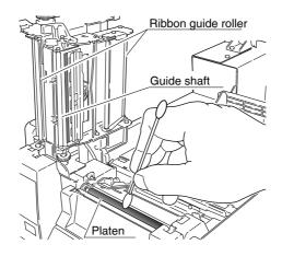
If the glue of the label media adheres to the roller, the peeled liner will stick and can cause a jam. Remove the glue adhered to the roller by using a cloth or something similar soaked in alcohol.
