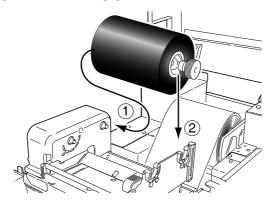
3. Push the large blue head-open lever to release the head unit. Pull out the ribbon from the bottom of the head unit to the ribbon winding side.
