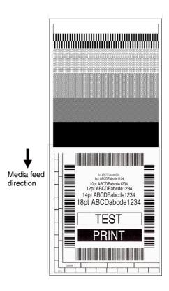
Using the Self Test Print shown above, you can make adjustments to the printer settings such as media width and media thickness (printhead pressure). For more details of the adjustment, refer to "4. Printer Adjustments."
