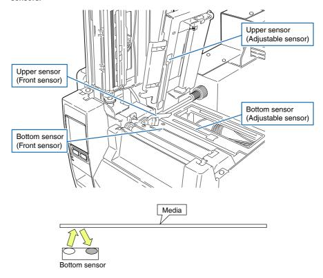
3. Adjust the sensors. Select "Reflect" from "Test & Info" on the menu screen -> "Test Mode" -> "Auto Calibration," and press the "OK" button at the bottom of the screen. Press the "Start" button on the screen displayed, and the sensor will be automatically adjusted.
