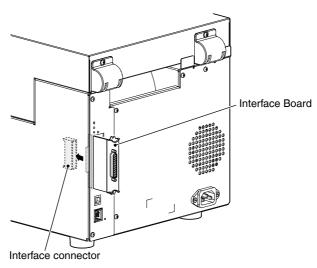
3. Fix the interface port to the printer by using the removed screw (2 nos).
