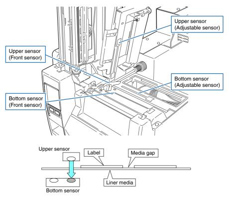
3. Adjust the sensors. Select "See Through" from "Test & Info" on the menu screen -> "Test Mode" -> "Auto Calibration," and press the "OK" button at the bottom of the screen. Press the "Start" button on the screen displayed, and the sensor will be automatically adjusted.
