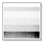
The first sample, left, shows an incorrectly set "media thickness adjustment". For standard label media, the media thickness adjustment indicator should be set to the center scale in the window.
