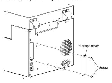
2. Insert the interface port into the slot, and connect to the interface connector inside the printer.
