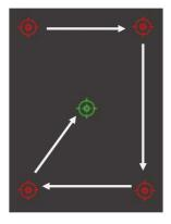
After touching all the targets, the following screen is displayed if the calibration is completed correctly. This completes calibration of the touch panel.
