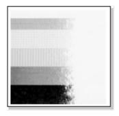
The second sample, left, shows an incorrectly set "media width adjustment". For 4-inch or 100 mm wide media, the adjuster should be set to the scale of 100 mm in the window.
