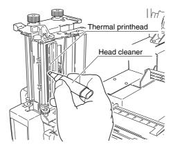
To clean the entire surface of the platen, rotate the platen little by little with your thumb using a cheese cloth. Do not touch the platen with your bare hands.
