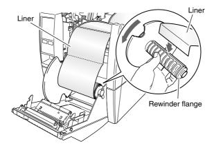
5. Confirm that the liner unit is in place in the peeler roller and close the rewinder cover.
