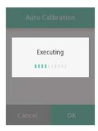
4. If the automatic adjustment is completed normally, "OK" will be displayed on the screen. If it is completed abnormally (adjustment not possible), the error LED flashes, and "Failed" will be displayed on the screen.
