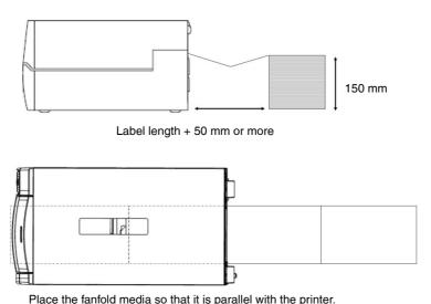
Insert the fanfold media through below media holder bar and set the holder by aligning it with the media width.
