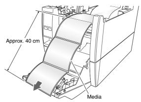
3. Peel off a number of labels at the tip part of the media from the liner so that the liner unit is in contact with the peeler roller when closing the rewinder cover.
