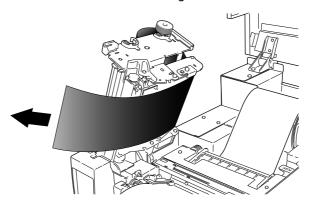
4. Using tape etc., fix the ribbon that you have pulled out on the ribbon holder on which the paper core has been set and wind it on the ribbon holder.
