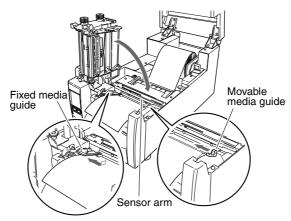
Lower the head unit back down to the closed position. Push the head close knob firmly to close and lock the mechanism.
