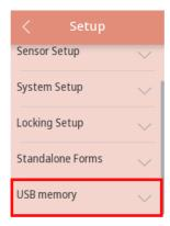
3. Press the "USB memory" button, and press "Update Firmware" from the expanded list.
