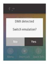
If "Yes" is selected, a restart is executed, and the printer automatically switches to Datamax® emulation (DM4/DMI/DPP).
