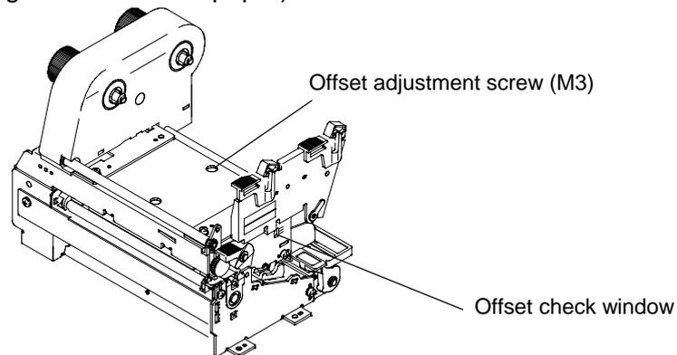
The relationship between the offset check window and the print head heating element is shown as follows:
