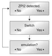
By selecting "Yes" the printer will reboot and automatically switch to ZPI2 emulation. The printer will return to the On Line Ready status if "No" is selected.
