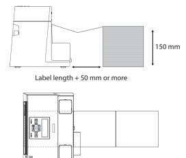
Place the fanfold media so that it is parallel with the printer.
