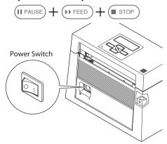
2. After "Sensor Cal Mode" lights up, release the keys to change the printer to sensor adjustment setting mode.
