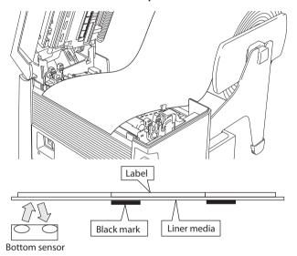
If the PAUSE Key is pressed then released while the MENU key is continually pressed, the sensor is automatically adjusted.
