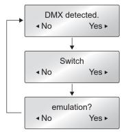
By selecting "Yes" the printer will reboot and automatically switch to Datamax® emulation (DM4/DMI/DPP). The printer will return to the On Line Ready status if "No" is selected.
