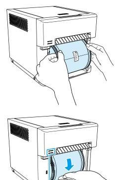
9 Remove the seal, place a hand on the paper, and rotate the paper holder in the direction of the arrow to insert the paper leading edge until the buzzer beeps.
