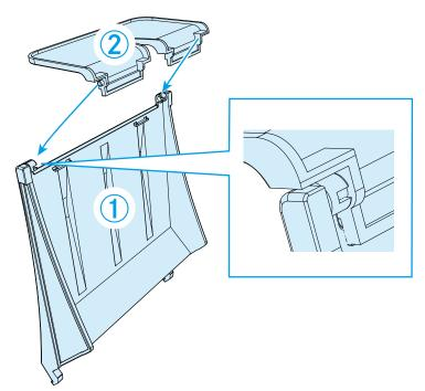
**2** Insert and push the pegs into the hooks.
