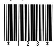
In a situation where the data " 1 2 3 " has been printed as code 39.
