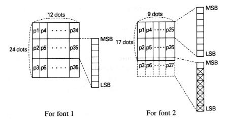
Each bit of the data is made up of '1' dots that will be printed and '0' dots that will not be printed.
