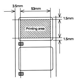
Note: Do not mix labels having different widths and length in the same roll of label paper.
