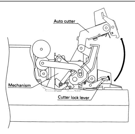
After closing the auto-cutter, check that the cutter unit is firmly fixed in the mechanism by the cutter locking lever. If the cutter unit is not firmly fixed, this will become a cause of paper jamming.
