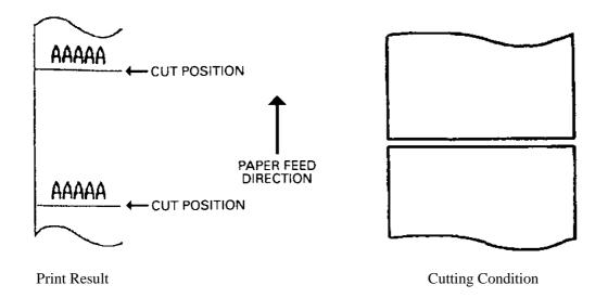
(42) Partial Cut (ESC m) (In selection of cutter option)
