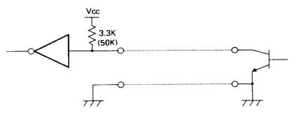
All the output signals are pulled up by  $50K\ Ohm.$
