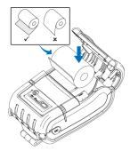
(2) Place the paper roll as shown. Make sure the paper is placed in right direction.
