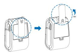
(2) Remove the battery as shown.
