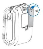
(2) Tighten the screw with driver as shown.
