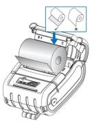
(2) Place the paper roll as shown. Make sure the paper is placed in right direction.
