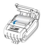
(3) Pull a short length of paper out of the printer and then press center of the paper cover to close the cover.
