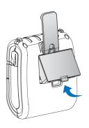
(2) Remove the battery as shown.
