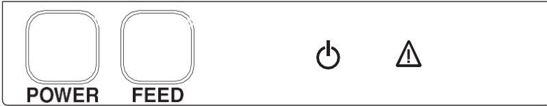
Two LEDs and two keys are placed on the operation panel.
