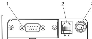
1. Interface connector (serial, parallel, USB, etc.)
