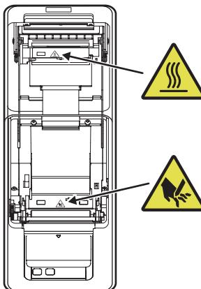
THIS LABEL INDICATES THE RISK OF BURNS DUE TO THE HIGH TEMPERATURE OF THE PRINT HEAD AND A RISK OF BEING CUT BY THE AUTO CUTTERS WHILE THE PAPER COVER IS OPEN.
