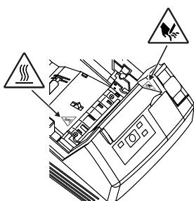
THESE LABELS INDICATE THE RISK OF ANY INJURY DUE TO "HIGHE TEMPERATURE" OF THE PRINT HEAD AND "SAW-TOOTHED EDGE" OF THE MANUAL CUTTER.
