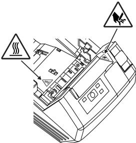
**THESE LABELS INDICATE THE RISK OF ANY INJURY DUE TO "HIGH TEMPERATURE" OF THE PRINT HEAD AND "SAW-TOOTHED EDGE" OF THE MANUAL CUTTER.**
