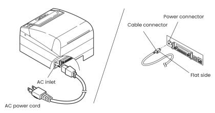
AC power type (built-in power supply) DC power supply type
