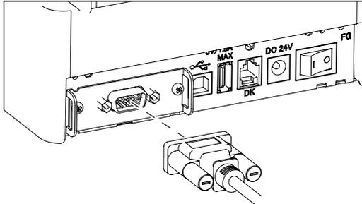
3. Insert the other connector firmly into the interface port of the host computer.
