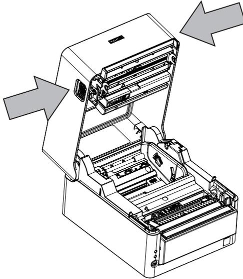
3. Load the roll paper with the printable side of the paper facing outward as shown by arrow A and with no slack.
