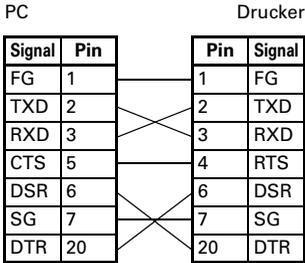
9-Pin – 25-Pin-Kabel
