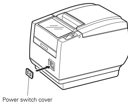
Put a screwdriver or other pointed object into the grooves on the power switch cover to remove it.
