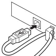
3. Insert the other connector firmly into the interface port of the host computer.
