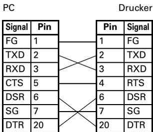
9-Pin – 25-Pin-Kabel
