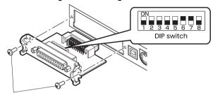
Serial interface board mounting screws
