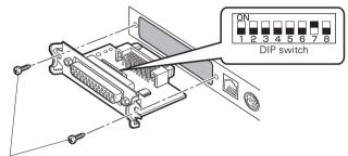
Serial interface board mounting screws
