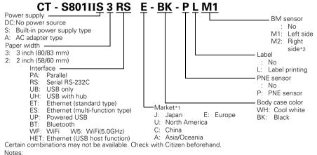
\*1: AC power cord, serial I/F screw, firmware and other specifications vary according to markets.
