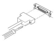
Insert the other connector firmly into the interface port of the host computer. 3.
