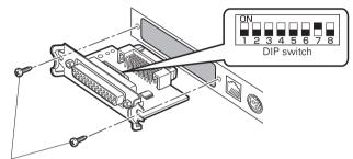
Serial interface board mounting screws
