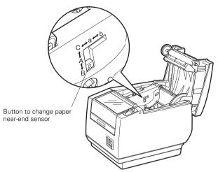
("A" and "B" are for horizontal installations, and "a" and "b" are for vertical or wall installations.)
