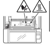
THIS LABEL INDICATES THE RISK OF BURNS DUE TO THE HIGH TEMPERATURE OF THE PRINT HEAD AND A RISK OF BEING CUT BY THE MANUAL AND AUTO CUTTERS WHILE THE PAPER COVER IS OPEN.
