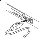
4. Secure the interface cable with the cable clamp.
