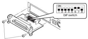
Serial interface board mounting screws
