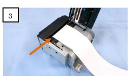
Put the roll paper in the place. (Paper leading edged to the arrowed position.)
