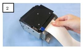
Insert the roll paper and push it until the leading edge hits the platen. And hold it awhile.
