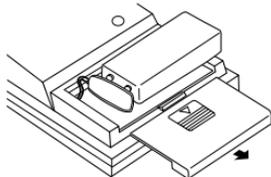
Take off the battery cover at the back of the unit by sliding it as shown.
